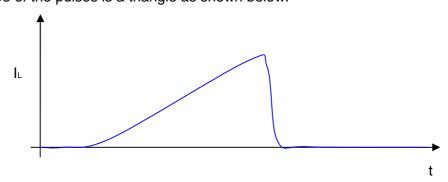
If the rms value of this current remains very low, the peak value may reach the tripping point of a magnetic circuit breaker if its range and curve type have not been well selected.
